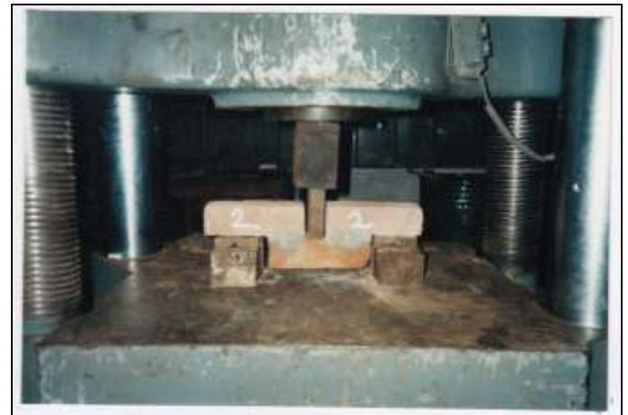
Figure 4. Mortar tensile test setup
