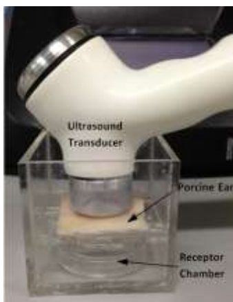
Figure 1. Representative photo of the experimental setup for using ultrasound in the transdermal drug delivery.
