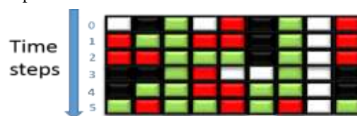
Figure 22: Example of one dimensional cellular automaton status after five step executions are completed.
