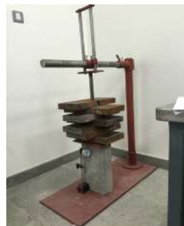
Figure 5. Experimental set up for creep test
