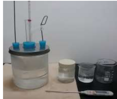
Figure 3 Photograph of freezing point measurement
