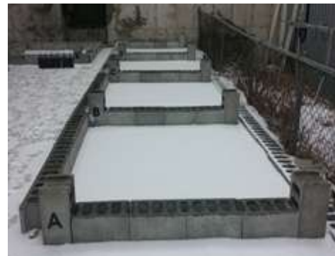
Figure 4 Photograph of snow melting performance test
