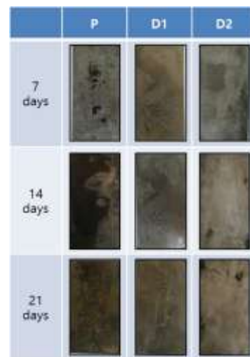
Figure 8. Steel corrosion by mix condition and age
