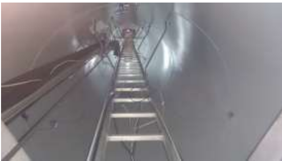
Fig. 7 Mounting accelerometers along the tower height.
