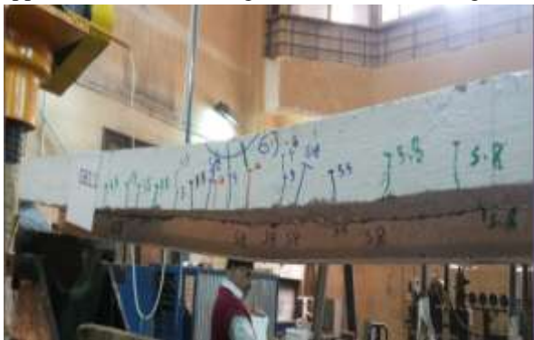
Figure (8): Crack pattern of composite beam GB1.1.
