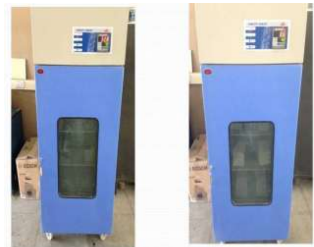
Figure 3. Specimens placed in humidity chamber to freeze and thaw cycle.
