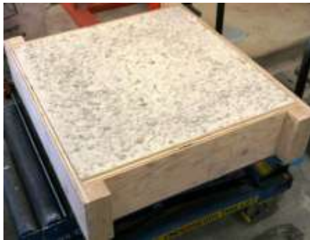
Figure 3. Casting of slab specimen
