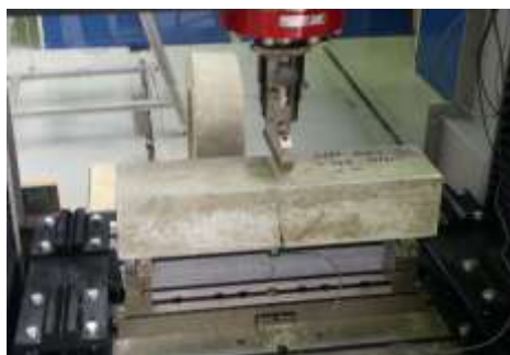
Figure 4. Three-point loading test of beam specimen
