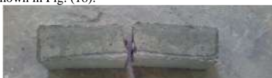
Figure 16. Fracture Shape (Brittle Failure) of PC Beam.
