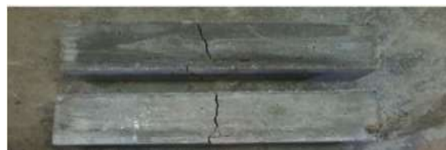
Figure 18. Failure Shapes for Bamboo Reinforced beams.
