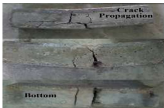
Figure 17. Ductile Failure of RCS Beams.
