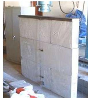
Figure 4. Wall section for axial compression test
