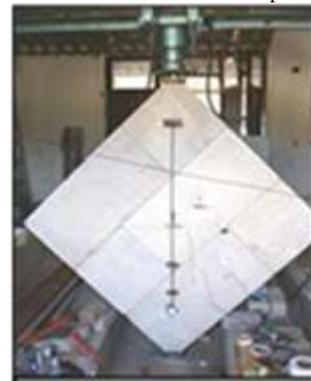
Figure 5. Wall section tested under diagonal compression
