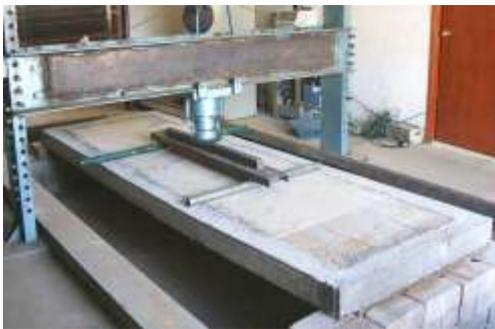
Figure 7. Roof section tested under two point bending test
