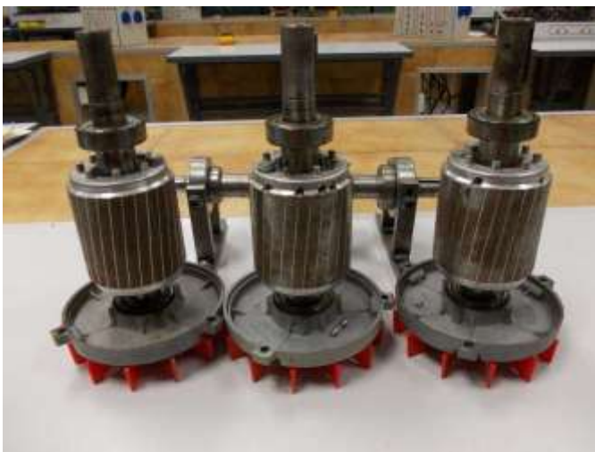
Fig. 4. Picture of the three rotors tested; healthy motor (left), motor with four broken bars (center), and motor with two broken bars (right).
