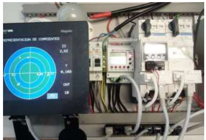
Fig. 5. Representation in the dartboard of the HMI from the two broken bar motor.
