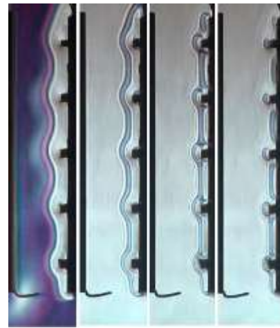
Figure 5. Schlieren images recorded with the focal filament progressively moved from its reference position in order to show the images of points of the optical field deflecting the light by the same known amount.
