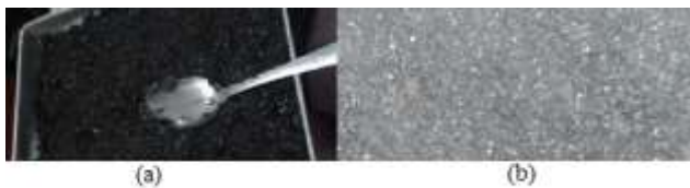
Figure 5 (a) Compost Char Paste, (b) Compost-Based Activated Carbon (CBAC)
