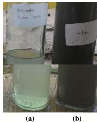
Figure 3 Comparison for Visual Turbidity of Samples; (a) AC Reactor and (b) Waste-Washing Wastewater (3W)
