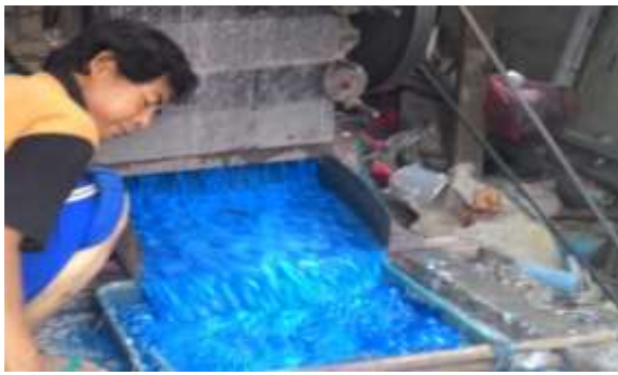
Figure 4 Waste-Washing and Grinding Process in MRF Zero Waste Indonesia (The Blue Colour is The Waste Being Washed)
