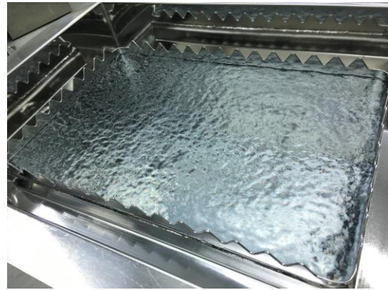
Fig. 1 Visualization of cavitation activity in 360/470 kHz multi-frequency megasonic system operating in thickness mode transducers
