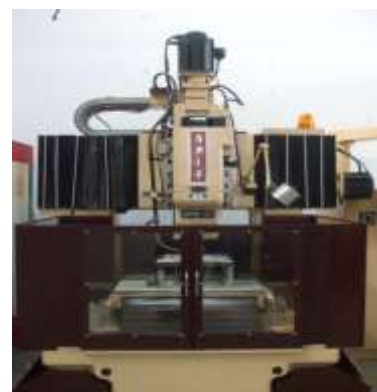
Figure 4: SPIF machine in DCSElab, C1 workshop of the Hochiminh City University of Technology.
