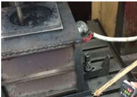
Figure 7: Heating system under SPIF feature 3
