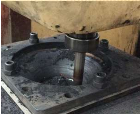
Figure 6: Forming Titanium model sheet by SPIF technology at 600°C with graphic powder lubrication
