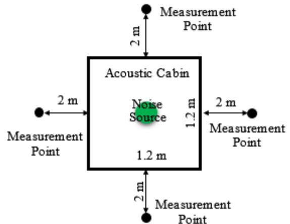
Figure 5. Measurement diagram
