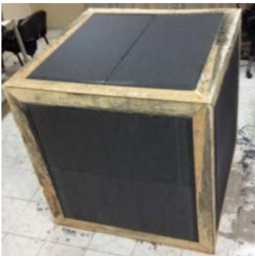
Figure 4. Styrofoam cabin
