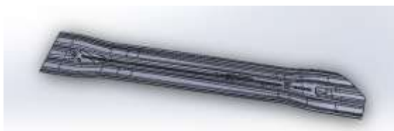
Fig.1 CAD model of Anti-intrusion bar
