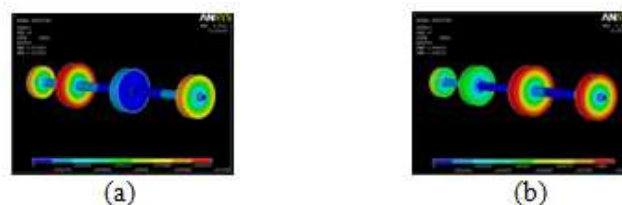
Figure 4. Mode shapes at torsional frequency (a) 20.008 Hz and (b) 30.001 Hz
