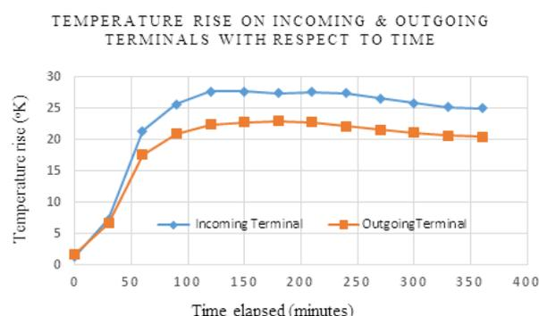
Fig. 7 Variation of Temperature rise with time elapsed for Incoming & Outgoing terminals of 66 kV isolator
