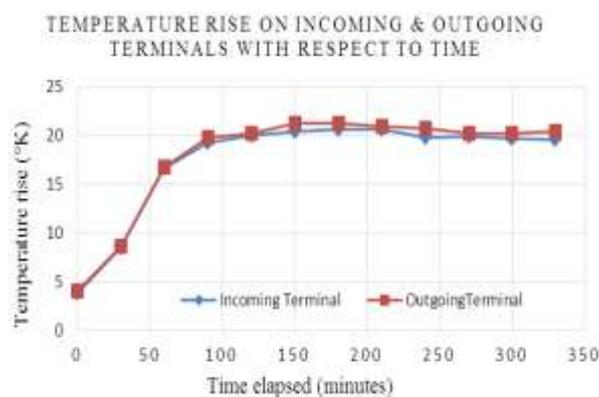
Fig. 10 Variation of Temperature rise with time elapsed for Incoming & Outgoing terminals of 220 kV Isolator
