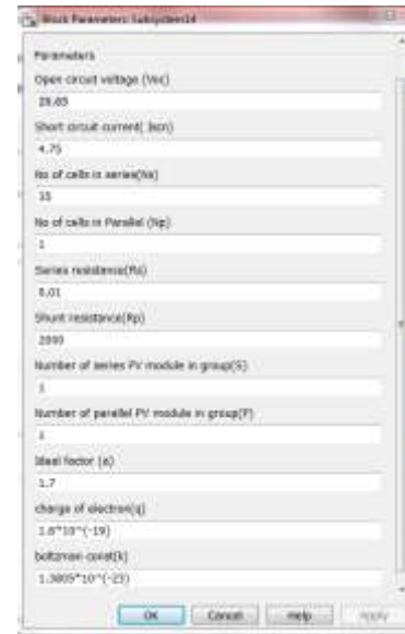
Figure 2 Masked PV model block parameter
