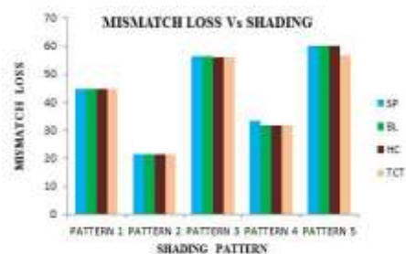
Figure 7 Mismatch losses for 4X4 array
