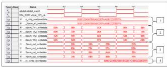
Fig.7. Screen Shot for SignalTap II Logic Analyser, when Parallel Ethernet Transceiver has been tested to transfer 128 bits
