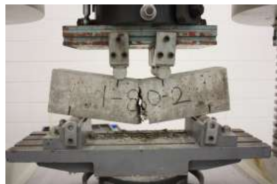
Figure 8. Flexural test of concrete with 3D fiber
