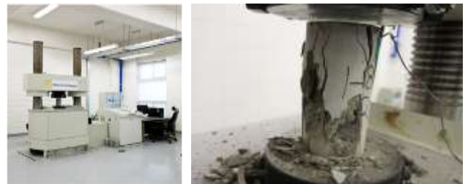
Figure 7. Compressive test of concrete with 3D fiber
