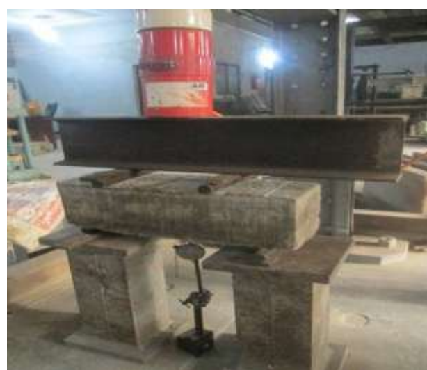
Figure 3. Flexural test of SCC beam specimens
