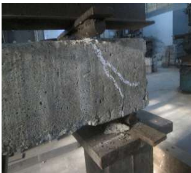
Figure 4. Failure pattern of tested SCC beams
