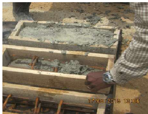
Figure 2. SCC beam specimen preparation
