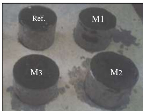
Fig. 2: Specimens used for measuring % chloride penetration
