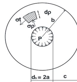
Figure 2. Concrete cylinder concentrically reinforced with FRP bar.
