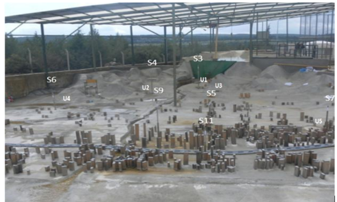
Fig. 9. Locations of the level meters (S1, S2, ..., S11) and UVP transducers (U1, U2, ..., U5)
