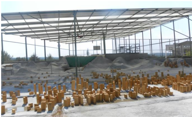
Fig. 6. The completed downstream part of the physical model
