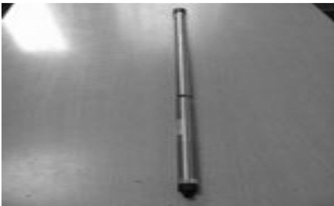
Fig. 7. e+ WATER L level sensors
