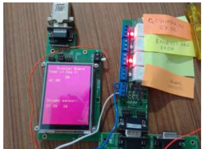
Figure 6. Operation of actuators AC &amp; oxygen cylinder
