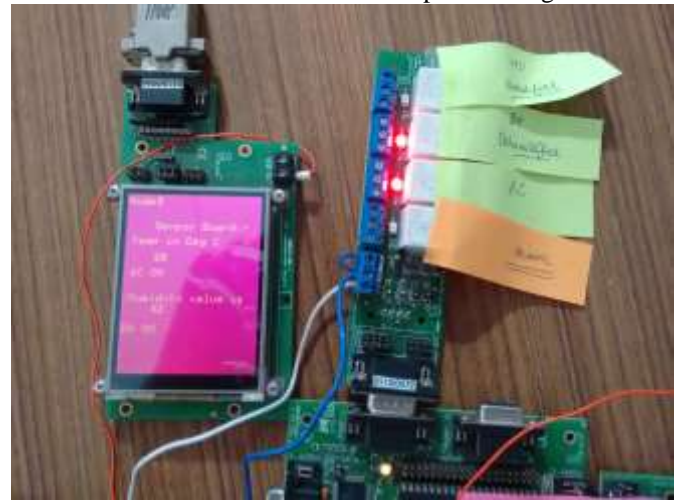
Figure 5: Operation of actuators AC &amp; dehumidifier
