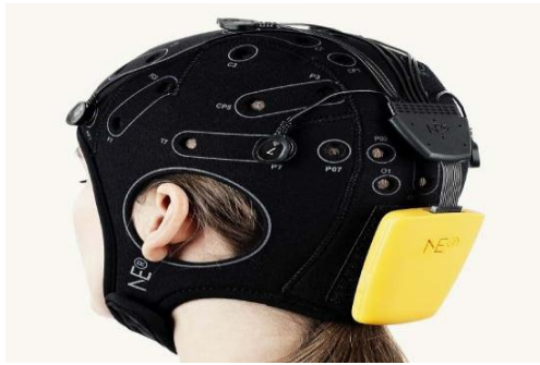
Figure 1: 8-Channel Enobio EEG Headset
