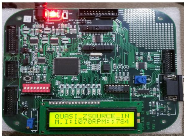
Fig. 9. Completed Controller Board for the Quasi-Z-Source Inverter
