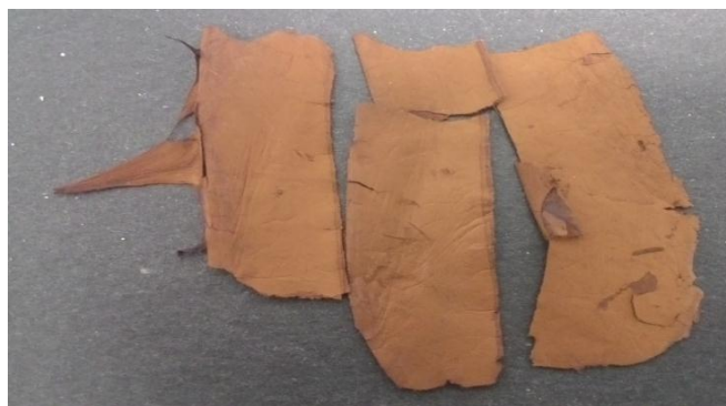
Figure-2. PAN nanofiber webs which were stabilized for 24 hours
