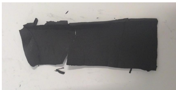
Figure-3. Stabilized PAN based carbon nanofiber which was carbonized in nitrogen gas for 45 min.
