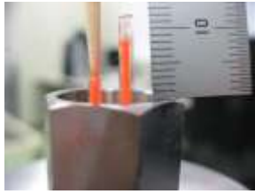
Fig.8 Measurement of liquid surface level
