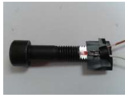
Figure 7. Strain gauge located at the stem
