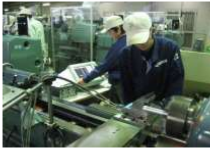
Fig. 11 Work come-off and fly-off experiment
