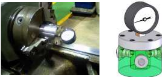
Fig.6 Measuring system for chucking force
