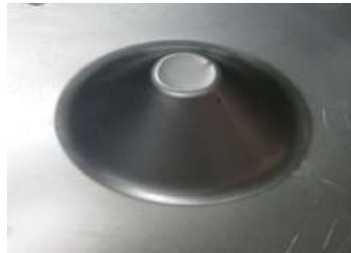
Figure 4. Formed conical part using SPIF
