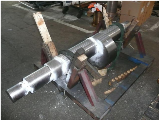
Fig. 4. Eccentric of the crank shaft with detected crack on the left side (clutch side)
