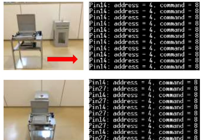
Figure 6: testing of the receipt of the Table id by robot
