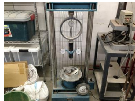
Figure 4 Penetration device used in CBR test
