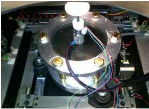
Figure 3. Inside view of the DIET clinical prototype, showing the actuator installed on the 2 – axis positioning system, while the breast interface mounted on the z-axis positioning motor can also be seen
