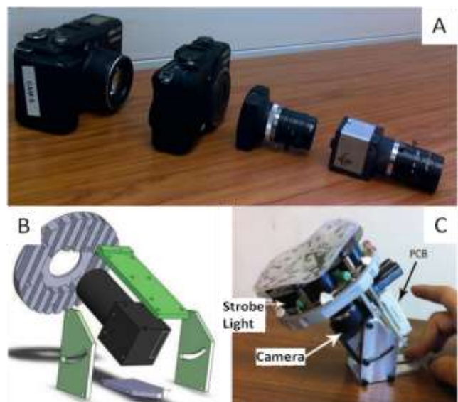
Figure 2. (A) Evolution process of digital cameras for DIET, starting from left Canon G5, Canon G9, IDS UI 1465 LE-C, IDS UI-2250 SE-C with C mount lens (B) Exploded view of the camera mount and heat sink (C) Assembled camera with strobe light and PCB ready to be mounted on the main frame Programming IDS UI 2250 SE-C
