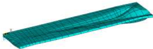
Figure 9. Geometry of wing profile – as imported from IGES file
