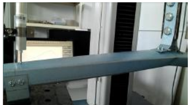
Figure 6. Deformation of the wall plate system
