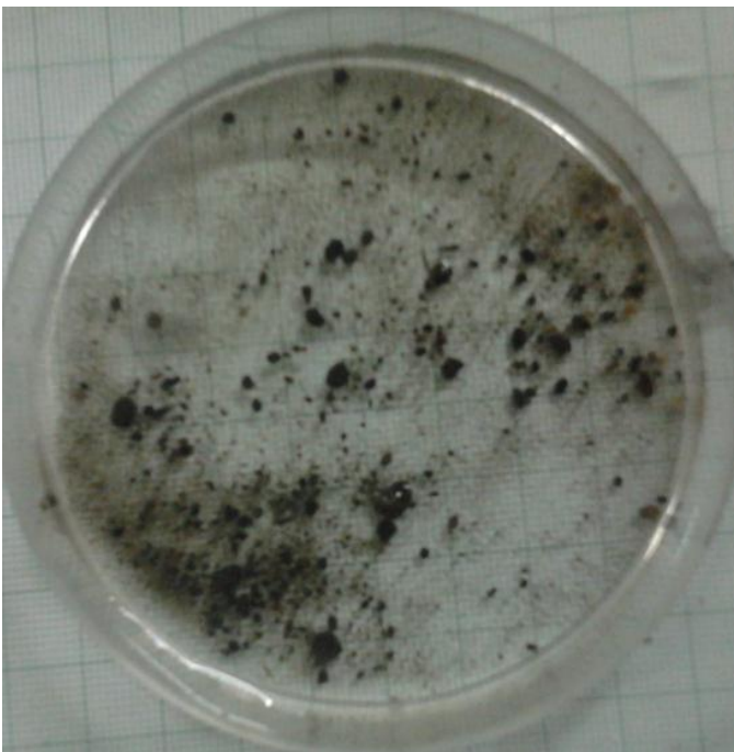
Fig. 2. Granules in EGSB reactor with chitosan
