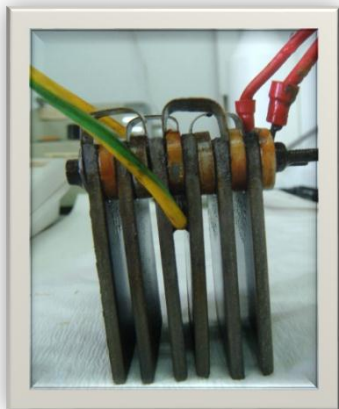
Figure 1. Aluminum electrodes in the parallel plate configuration used in the experiments.
