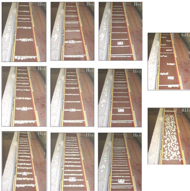
Figure 1. Tested macro-scale roughness configurations: transversal stripes (different boulder sizes and spacings), groynes and random arrangements.
