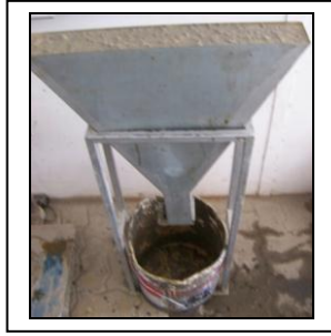
Figure 3. Experiment in progress for V-funnel test
