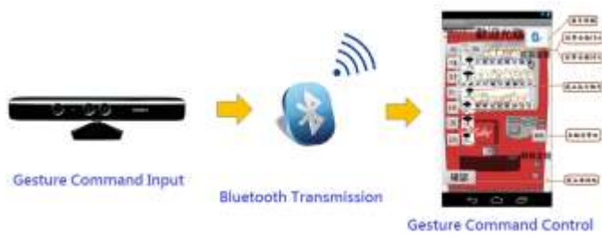
Figure 4. Kinect-captured gesture command made by the user for controlling the android application of vending machines through the Bluetooth wireless transmission.
