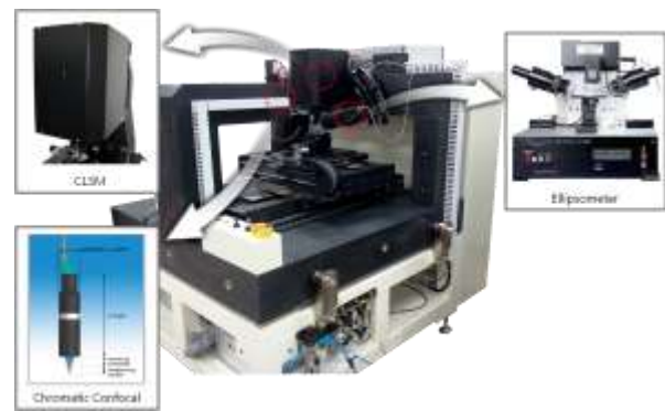
Fig. 10 Multi probe layout of measurement system
