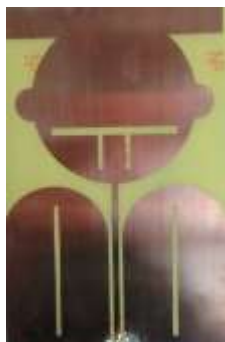
Figure 11. Printed circular coplanar patch antenna with connector soldered to the port
