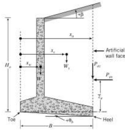
Figure 1. a typical rigid cantilever retaining wall [7]
